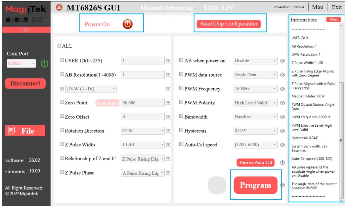
Figure 4.1.6 The interface state after chip power on
