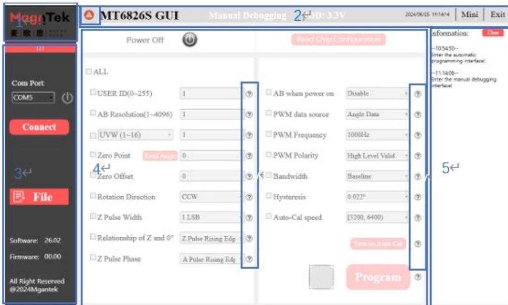
Figure 3.1.2 MT6826S Manual Debugging Interface
