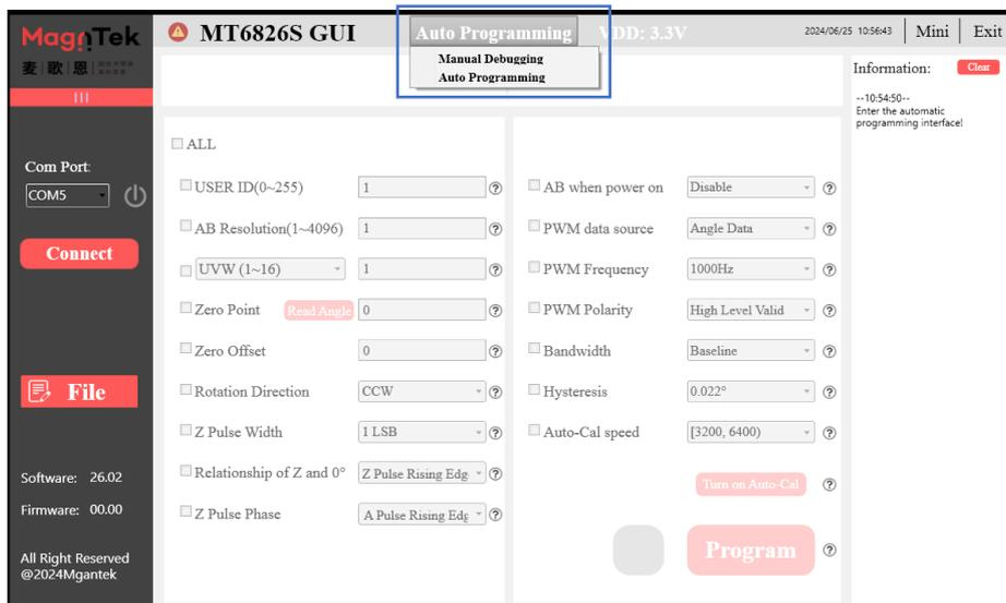
Figure 3.1.1 Program Interface Switch Selection
