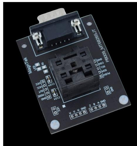
Figure 1.3 PB009-MT626SJT Socket Adapter Board
