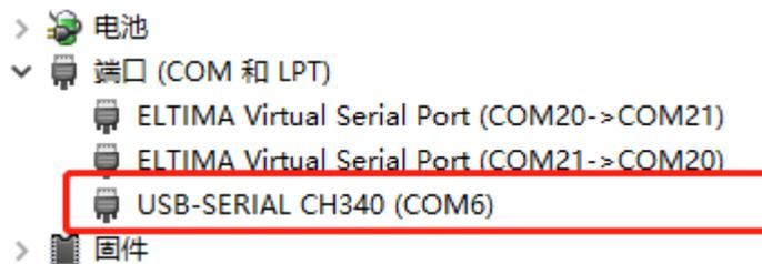
*Figure 2.1 Driver Successful Installed and Plugged to Programmer*
