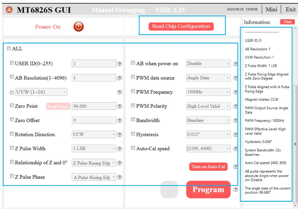
Figure 4.1.7 Read Chip Configuration
