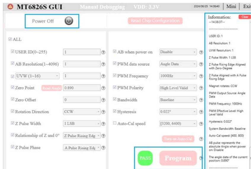
Figure 4.1.12 Software interface after chip power down
